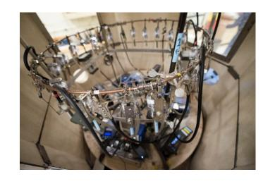
Even for factory-calibrated respirable dust monitors, the response to different dusts can be quite different
