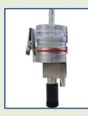
A novel sampling cassette was designed to facilitate the analysis and minimize losses (user friendly)
