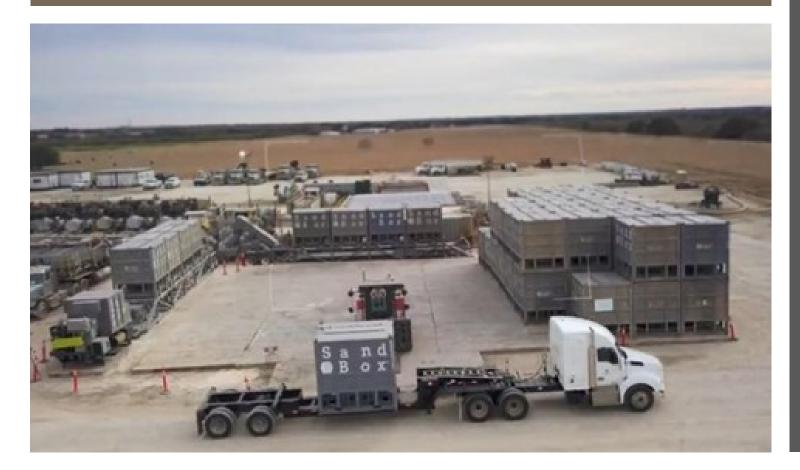
Hydraulic fracturing using Containerized Sand System
