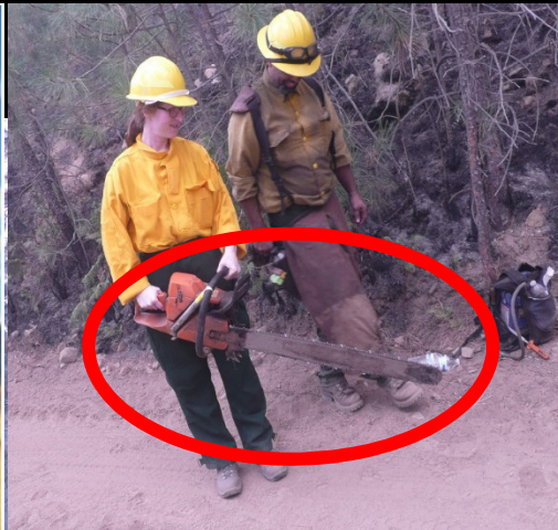
Chain saw with 4 ft. blade \approx 20 lbs.
