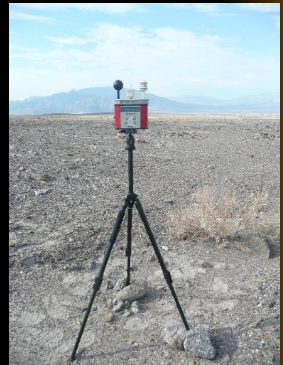
Wet bulb globe thermometer (WBGT) placed at each work location
