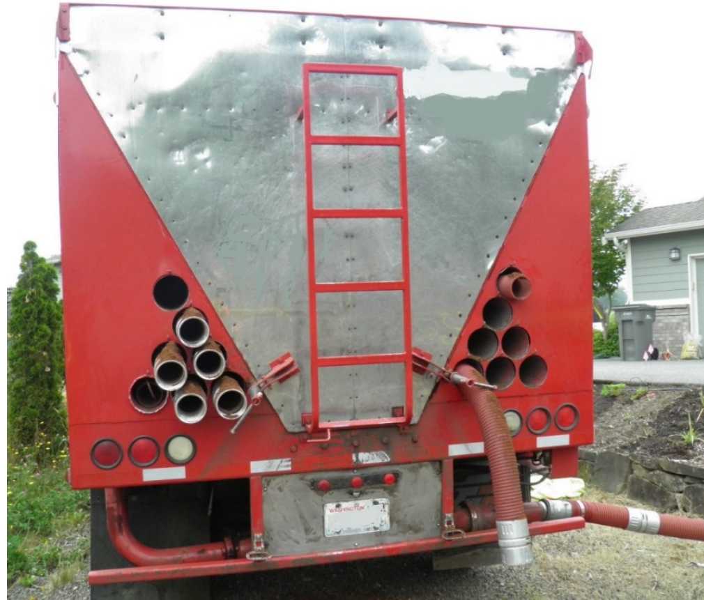
Rear of the bark blower truck with the hopper access ladder and hose assemblies.
