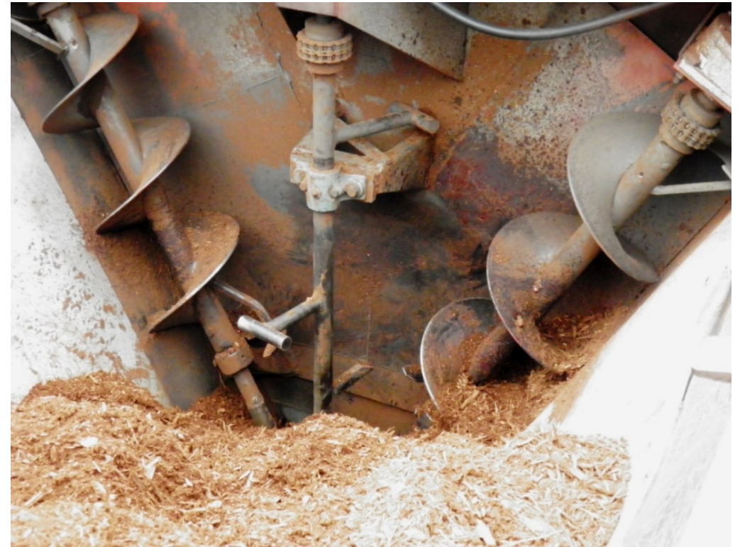
The auger system used to deliver bulk material into the feeder mechanism located on the cargo hopper bed. The auger system is located on the rear interior of the bark blower truck.
