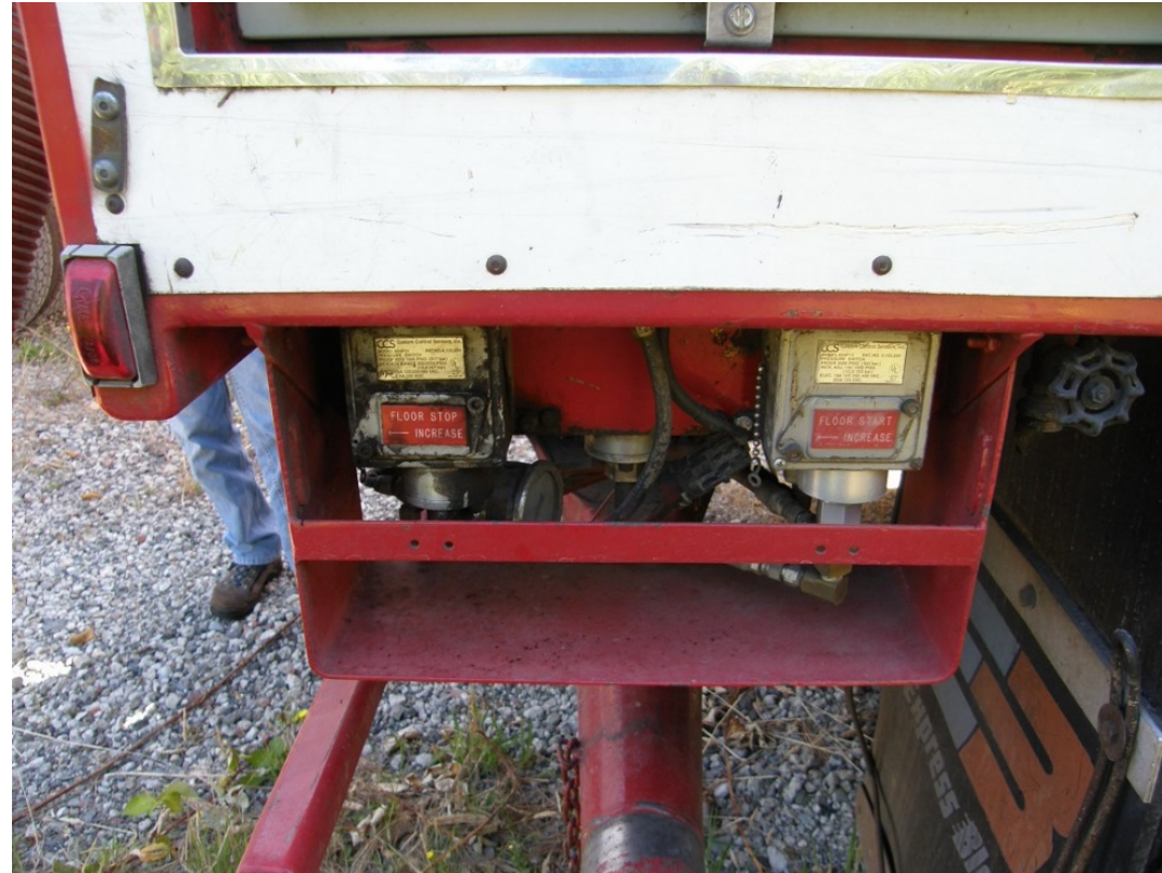
Pressure control switches on bark blower truck that were not operative and for which employer could not find replacements.
