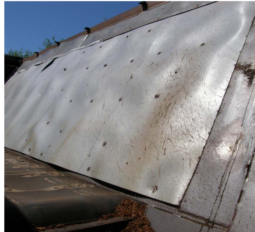
Interior wall of the bark blower truck's hopper. Scratches on the rear of the wall near the auger system may have resulted from pitch forks used by employees to feed bark into the blower system while standing on the bark.
