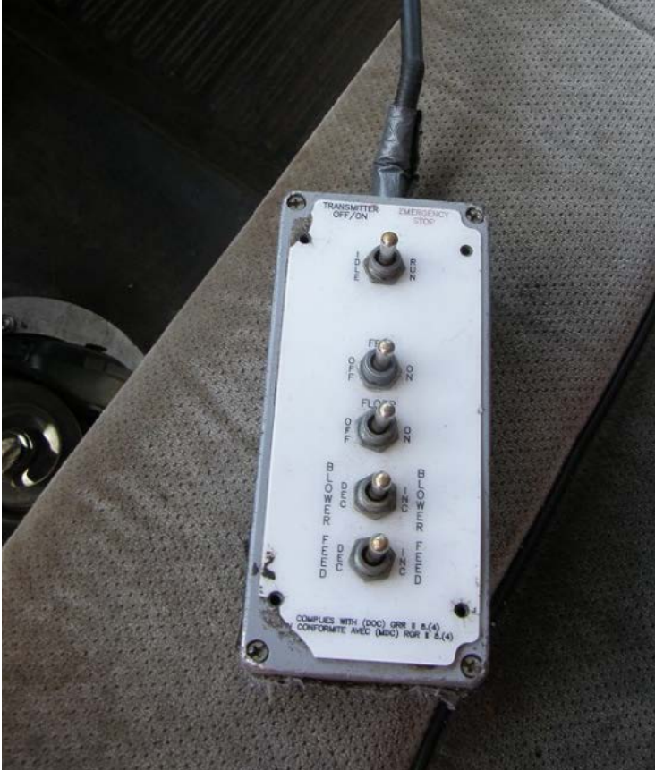
Remote control used by the crew leader to operate the blower system.
