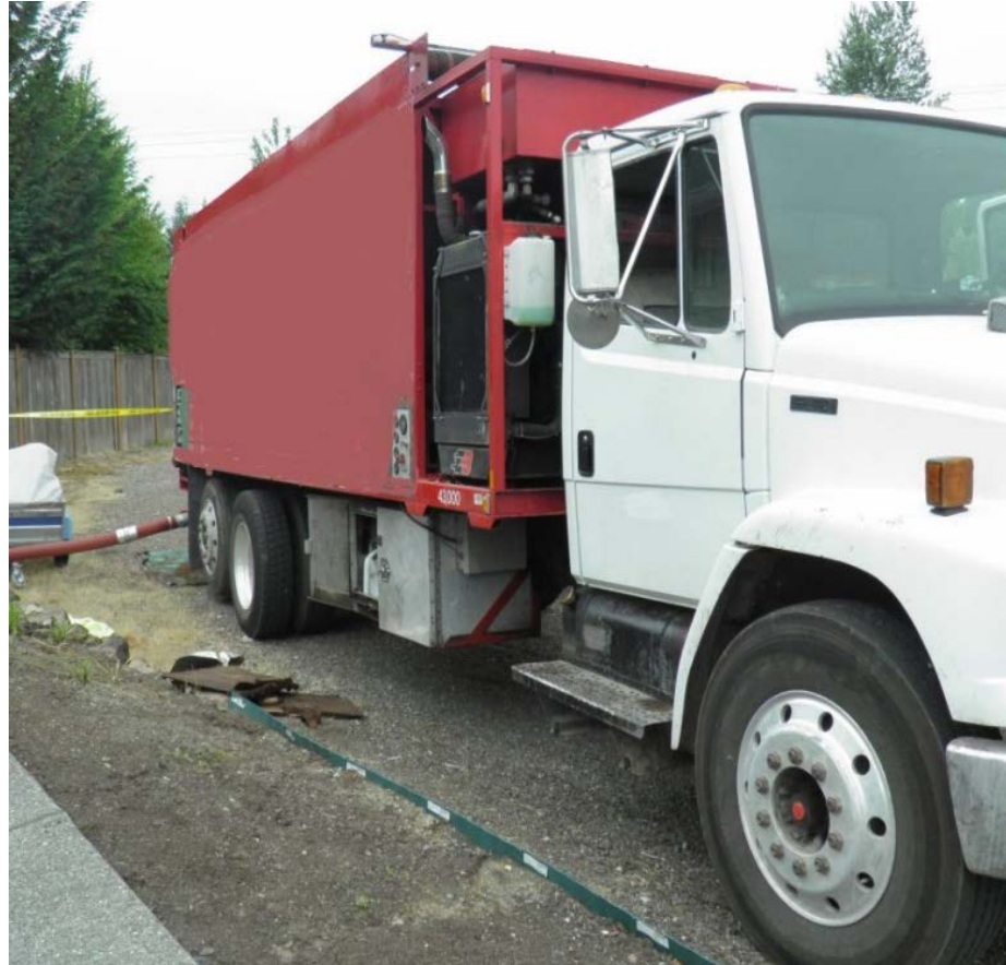
Bark blower truck at the incident site. The victim was working inside the cargo hopper near the rear of the truck. The delivery hose can be seen extending from the rear of the truck.
