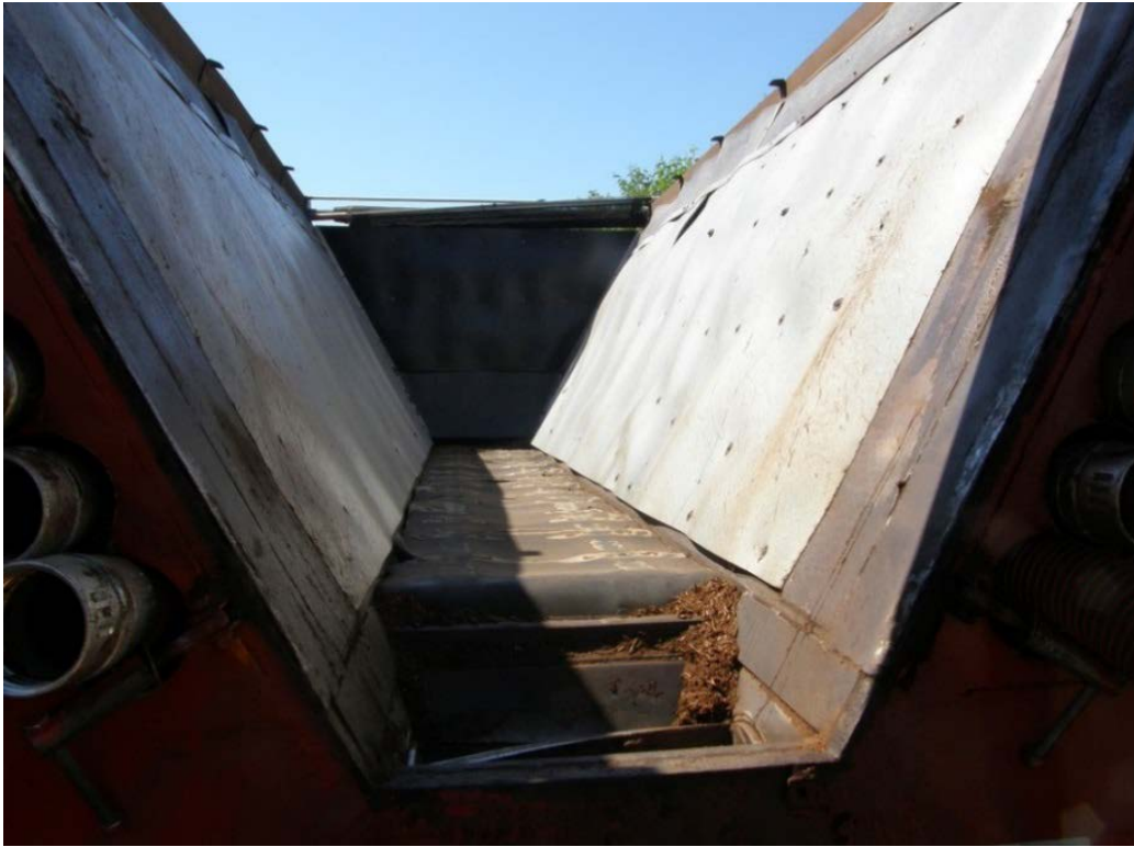
The empty cargo hopper of the bark blower truck. The material conveyor belt and feeder mechanism can be seen on the hopper bed.
