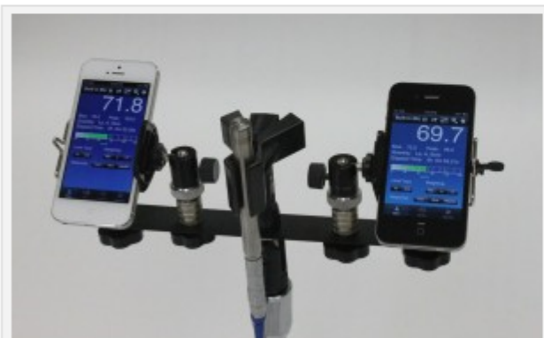
Figure 1. The SoundMeter app on the iPhone 5 (L) and iPhone 4S (R) compared to 1/2" Larson-Davis 2559 random incidence type 1 microphone (C).
