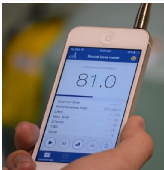
Image of the main screen of the NIOSH SLM app (shown with a MicW i436 external microphone)
